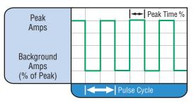
In excess of 40 PPS, Pulsed TIG becomes more audible than visible — causing increased puddle agitation for a better as-welded microstructure.
