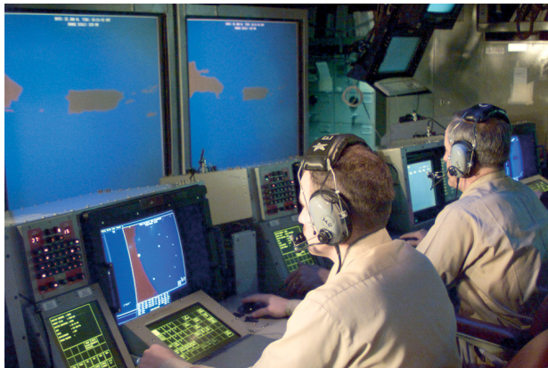
Figure 2. The Combat Information Center aboard USS Vicksburg (CG 69), an Aegis Baseline 6 Phase I cruiser. Shown is the ADS, which is directly based on APL's CDK Version 3.0. All ADS consoles and large-screen displays use CDK software and also incorporate many CEC display functions.
