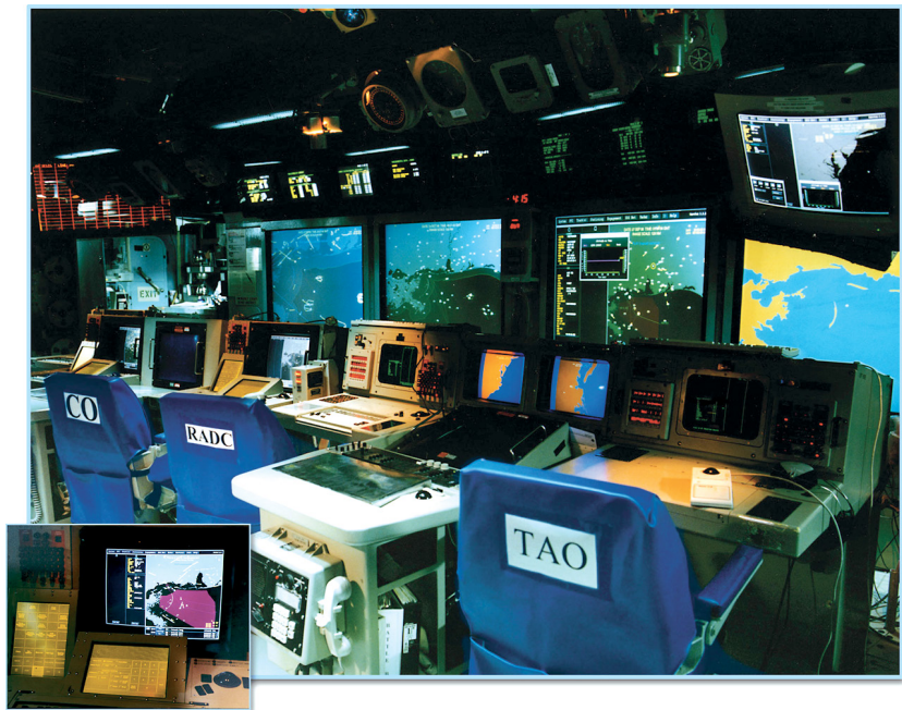
Figure 1. The Combat Information Center aboard USS Cape St. George . Two APL prototype displays are shown alongside the Baseline 5 ADS. A CEC display can be seen on both a 21-in. monitor and on large-screen display #3 (second from the right). The CDCS occupies large-screen displays #1 and #2 as well as the Commanding Officer's console (inset). Other displays are ADSs.
