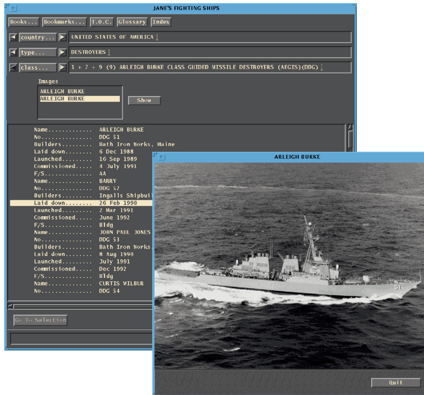
Figure 6. The Jane's database browser. The various Jane's books were selected for prototype online intelligence database applications. The browser, especially designed for CS@SE, provided a unique hierarchical browsing mechanism, bookmarks, simplified hyperlinks, keyword searching, and indexing. Text was stored on display hard drives, but images remained on CD-ROMs because disk space was a scarce commodity in the early 1990s.
