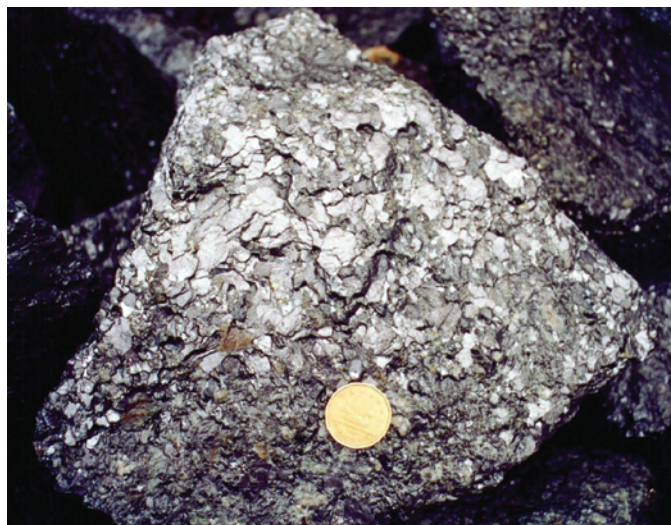
Figure 13. Massive hemo-ilmenite ore from the floor of the Main pit at the Lac Tio deposit, Quebec. Coin used for scale is about 26 mm in diameter. Photograph provided by Serge Perreault, used with permission.
