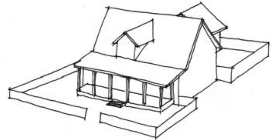
Acceptable Fence Locations: Fences bound yard areas, return into buildings, and stop where structures are near property edges.
