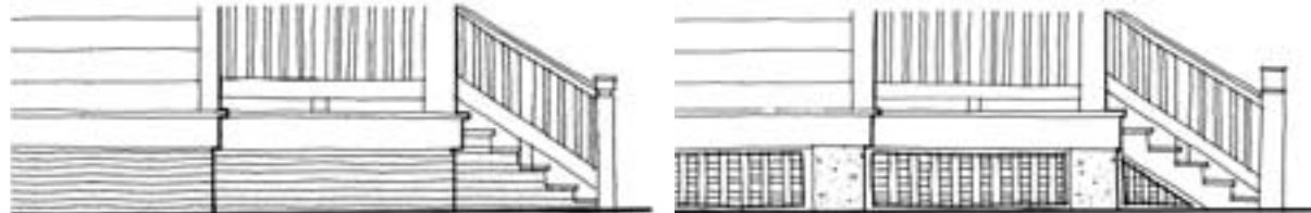
Continuous brick base.
