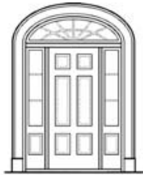
Six panel door with side lites and ellipse transom. Casing is substantial in width with back band edge.
