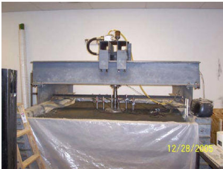
Figure 2. Laboratory test setup for full scale stabilization study
