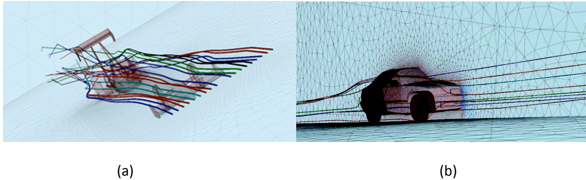
Figure 2. Distributed streamlines calculation and visualization for (a) a drag racer vehicle and (b) a BMW315 sedan.
