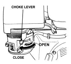
Figure 5. Choke Lever
