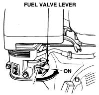
Figure 4. Fuel Shut-OFF Lever
