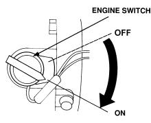
Figure 7. Engine ON/OFF Switch
