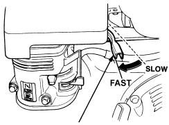
THROTTLE LEVER Figure 6. Throttle lever Lever
