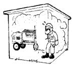
narrow area where free flow of the air is restricted. If the air flow is restricted it will cause serious damage to the mixer or engine and may cause injury to people. Remember the mixer's engine gives off DEADLY carbon monoxide gas.
