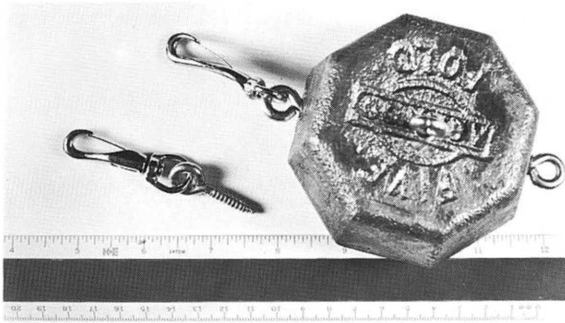
Figure 2. A 5-lb lead ingot ready for installation.
