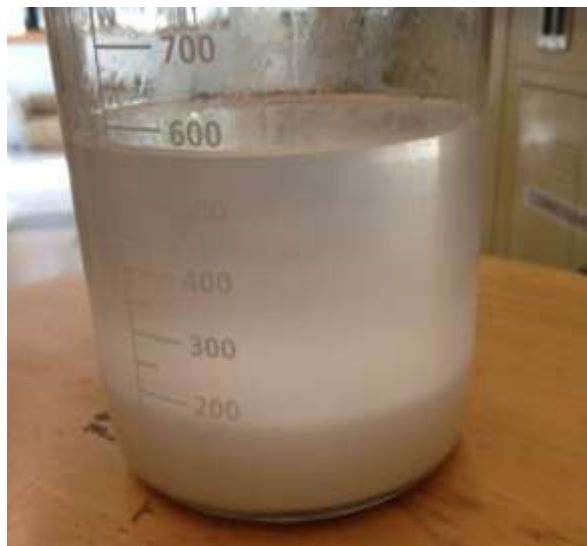
Figure S13. Large scale synthesis of UiO-66 made via the HCl-containing procedure presented herein.
