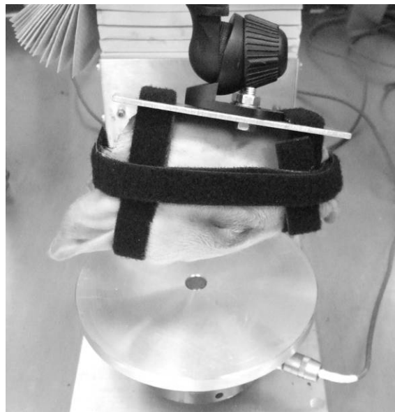
Figure 12. Picture of pig attached to mounting rod with straps.
