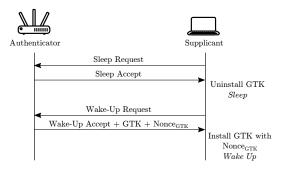
Figure 6: WNM Sleep Mode: Typical Message Exchange.
