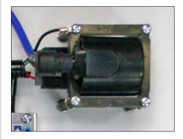
The one component in the modern ignition system that virtually all systems have in common is the ignition coil. If a student understands what happens in this component, he will understand ignition systems.
