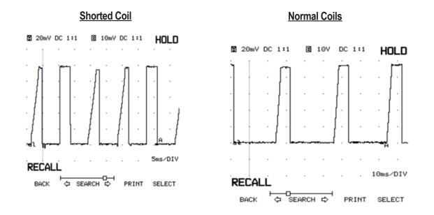
If a shorted or open coil is present the normal pattern will not be seen. Instead for a short, the pattern will go straight up and with an open it will stay at zero and leave a gap in the pattern. This pattern also shows a flat top of the coil current, so the current limit function of the module is present.
