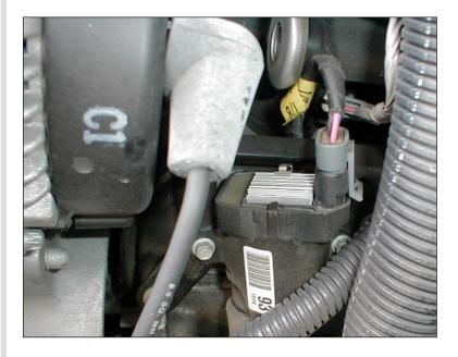
Some coils that are in the DIS category will have a heat sink showing. It allows the module which is contained within the coil to keep cool. The picture is from a GM vehicle. The silver finned object on top of the coil is the heat sink.
