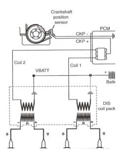
Notice that the PCM is functioning as the ignition module controlling primary current to each coil individually. A CKP is being used as the input device for speed and position. On these systems it is virtually impossible to capture a primary voltage waveform, so primary current is used. It can be used to compare each coil. Control the time/Div so the number of pulses on the screen slightly exceed the number of coils.
