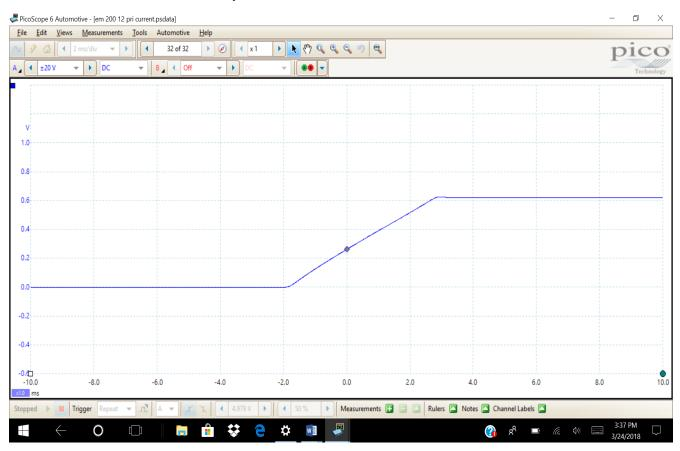
On the left is 0 amps. Once the difference between the two terminals of the coil is full voltage, current will ramp or increase from 0 to about 6 Amps. In this example we are using an amp probe that generated 100 mV for every amp flowing. We are right at 600 mV or 6 amps flowing. Take your time with this since an understanding of voltage drop causing current flow is fundamentally basic to their understanding of just about everything.
