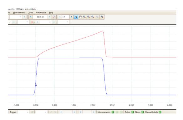
At idle the current ramp shows 3 pulses to charge the coil and fire it 3 times. This pattern is at idle. Once the engine is above about 1000 RPM the pattern shows (on right) that the coil is being charged once and discharged once. This is done for emissions which are typically higher at idle. A multi spark discharge tends to get more of the A/F ratio burning.
