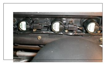
There are some systems that use a multi spark configuration. This Ford Coil On Plug system will fire the plugs multiple times at idle and switch over to a single firing once the vehicle is above idle (about 1000 RPM). The patterns for this system will confuse students and beginning technicians so make sure you go over them toward the end of the unit.
