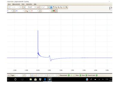
Placing the probe on an ignition coil of a Ford TFI ignition system produced the following pattern. The spike tells us that a spark did occur and the horizontal line (burn time) tells us how long it sparked. The scale at the bottom or the screen can be interpreted to give burn time, but an easier method is to use cursors.
