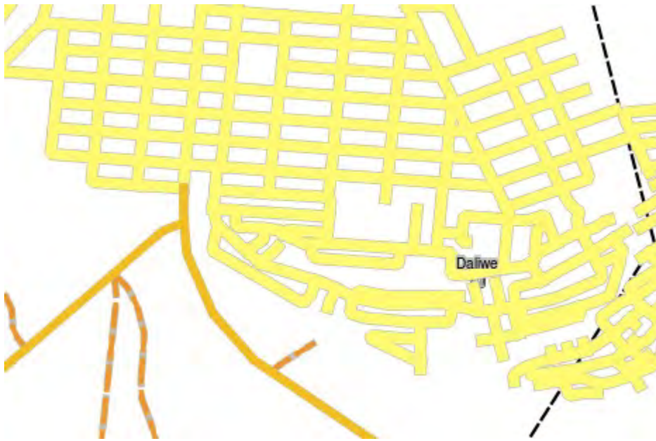
Illustration 42: A roads vector layer symbolised using a unique value per road type.
