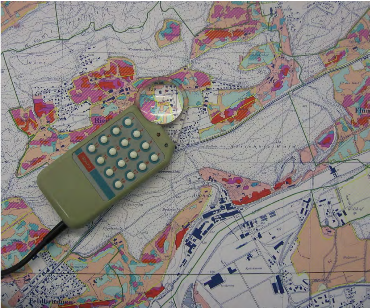
Illustration 50: A digitising table and puck are used by GIS professionals when they want to digitise features from existing maps.
