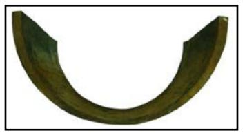
Figure 1: 65% thickness reduction of a 20-in. diameter carbon-steel pip after nine months of operation.
