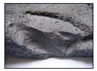
Figure 4: Pitting and craters on the damaged surface.
