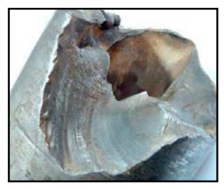
Figure 7: Step pattern fracture zones in the failed upper drive shaft.
