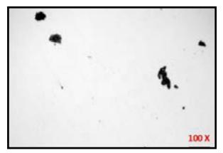
Figure 8: Observed nonmetallic inclusions.
