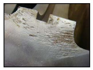
Figure 2: Erosion wear, pitting, and cracking in the pump casing of a lean-solution pump.
