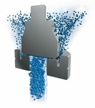
Homogenizing valve: the particles are pushed through a very narrow orifice by the high pressure and are smaller when they exit
