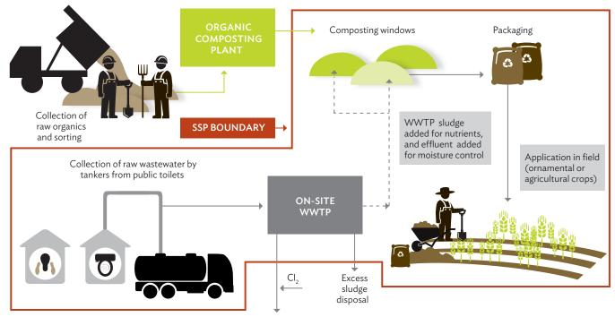
Figure 1.1: Sanitation Safety Planning System Boundary of a Wastewater Treatment Plant in Viet Nam
