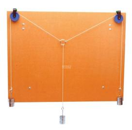
probably due to some hidden friction force that prevents the strings moving quite freely. Check that the pulley-wheels spin easily, and that the weights don't rub against the board.
