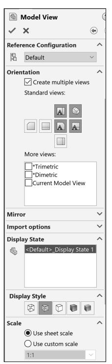
9) Notice that the isometric pictorial is very large. So, the size needs to be reduced. Select the pictorial view in the drawing area and set the display style as Shaded with Edges and use a Use custom scale and a 1:2 scale.
