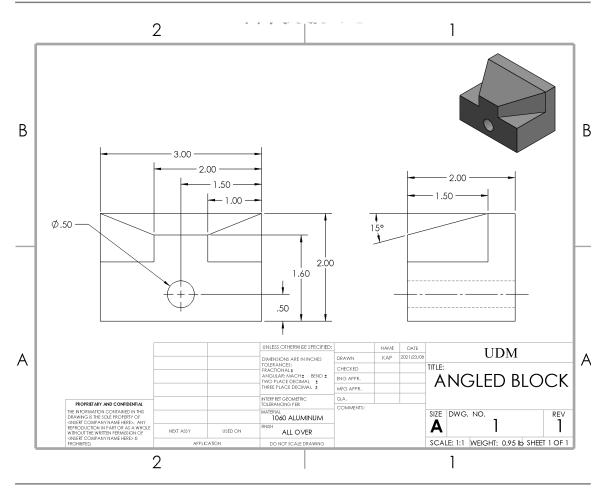
Figure 2.6-1: Angled block detail drawing
