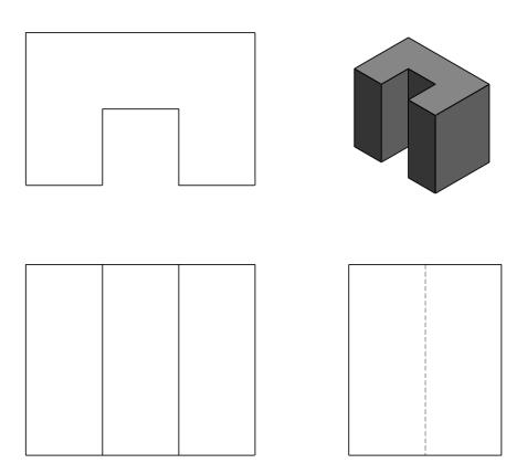
Figure 2.7-1: U-Block initial orthographic projection
