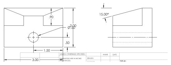
2) The *Front* view will be focused on first. Click and drag the dimensions to the approximate locations shown in the figure. If a dimension is not currently in the front view, click on the dimension, hold the **SHIFT** key down and drag it to the front view.
