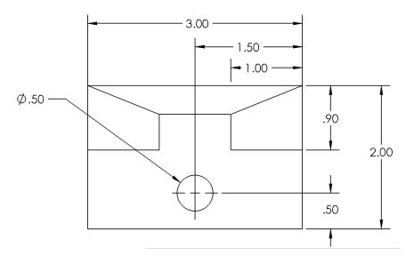
3) Delete the .90 dimension and add the 1.10 and 2.00 dimensions using Smart
