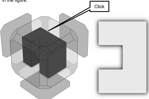
3) Notice that the view is not in the correct orientation for the *Front* view. Hold down the **SHIFT** key and then hit the **Left arrow – Up arrow – Right arrow** in sequence. This should place the view in the proper orientation. If it does not, continue figuring out the proper arrow sequence until the *Front view* looks like the figure.
