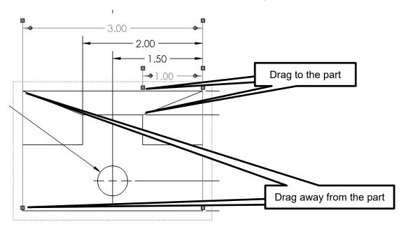
8) Drag the dimensions and the dimension text into the correct locations. Holding the **ALT** key will produce a smooth drag. The final *Front* view should look like the figure.
