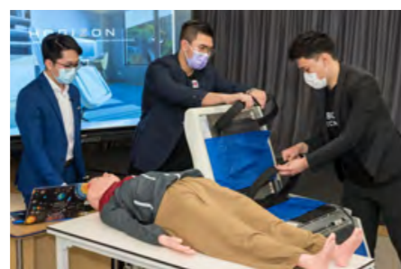
HORIZON, a smart patient transfer robot based on concepts conceived for a transformable wheelchair that extends horizontally.
