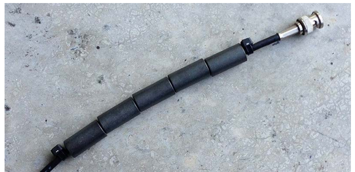
Figure 13 – Five ferrite cores secured with wire zip ties at antenna connector end of coax feed line.
