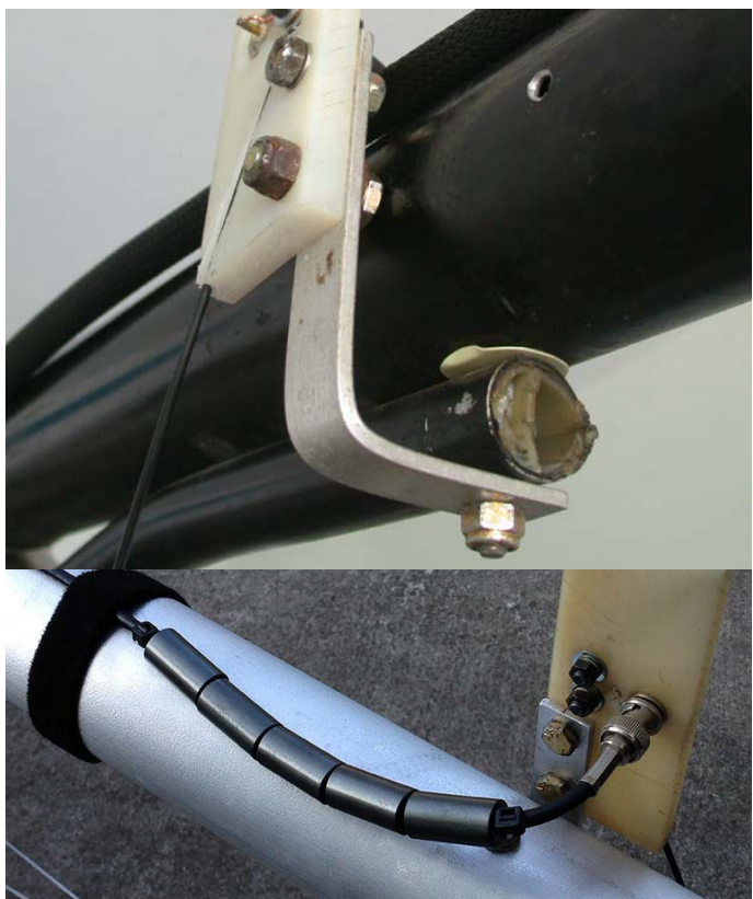
Figure 14 – Antenna mounted using an L-bracket. Anything similar will work as well.
