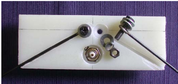
Figure 8 – Mounting the antenna elements and BNC connector.
