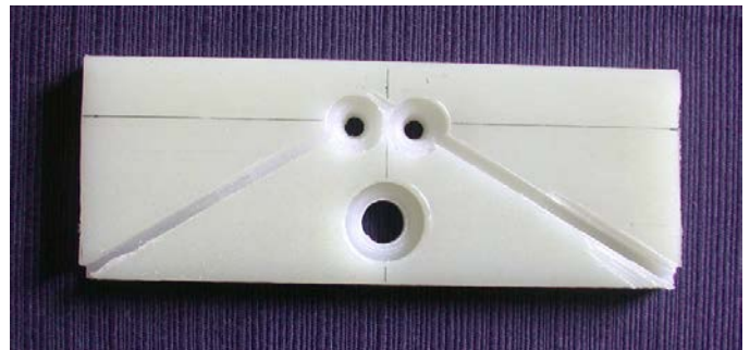
Figure 7 – Grooves for antenna elements cut into block.
