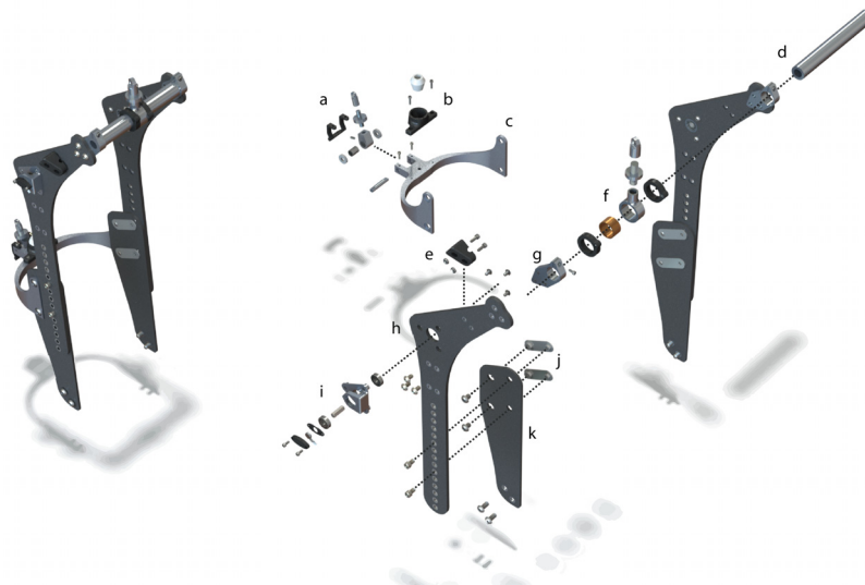
Fig. 7. Shank segment of the exoskeleton. Assembled (left) and exploded (right) views of the shank segment of the exoskeleton. (a) Knee flexion load cell assembly. (b) Ankle Bowden cable attachment. (c) Calf cuff. (d) Knee extension crossbar. (e) SLS nylon hard stop. (f) Knee extension load cell assembly. (g) Knee extension clamp. (h) Upper shank strut. (i) Knee joint assembly. (j) Threaded inserts. (k) Lower shank strut.
