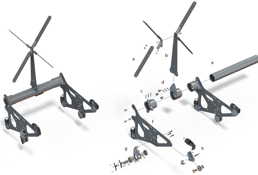
Fig. 5. Torso segment of the exoskeleton. Assembled (left) and exploded (right) views of the torso segment of the exoskeleton. (a) Shoulder strut. (b) Back strut. (c) Lateral back crossbar clamp. (d) Medial back crossbar clamp. (e) Back crossbar. (f) Waist strut. (g) Hip joint assembly. (h) Pulley assembly.
