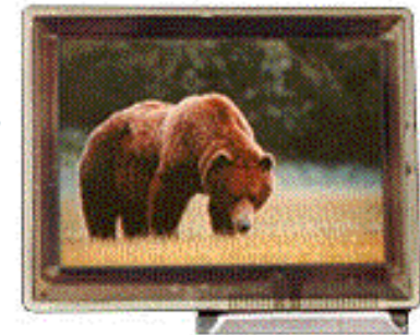
Sanyo Color AMOLED display - 852x222 pixels (prototype, 2.5" diag.) A 5-inch QVGA has also been shown
