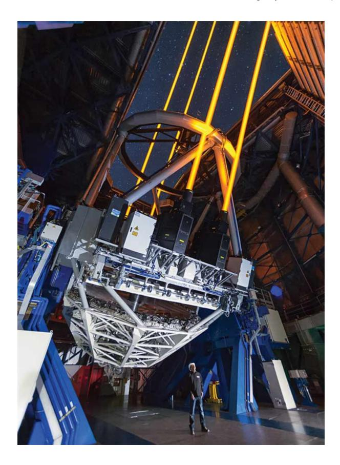
Four lasers excite sodium atoms and create artificial stars, 90 km up in the atmosphere, for the European Southern Observatory's Very Large Telescope's adaptive optics systems. Courtesy of European Southern Observatory.
