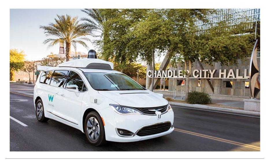
A self-driving car equipped with radar, lidar, and other sensors for navigation. Courtesy of Waymo.
