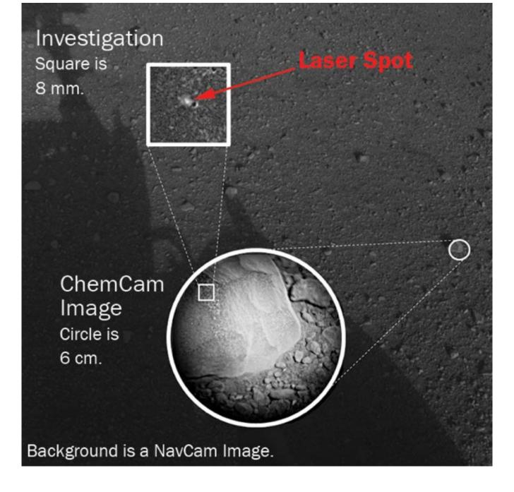
The Mars rover Curiosity zapped a rock with a laser, enabling spectroscopy to determine the rock's composition. Courtesy of NASA.
