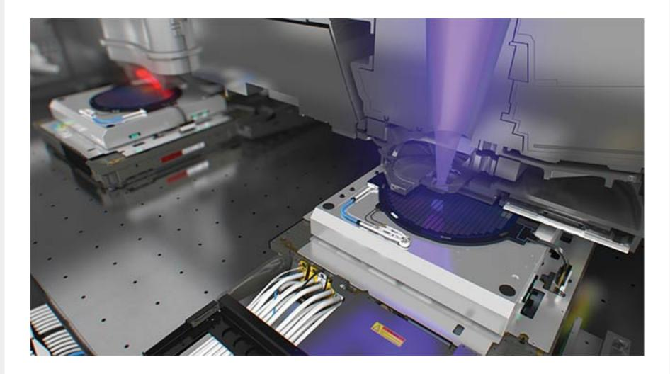
A critical step in manufacturing, semiconductor lithography uses lasers, as shown in this rendering of the exposure and printing of EUV (extreme ultraviolet) lithography of a semiconductor wafer on a stage. Courtesy of ASML.
