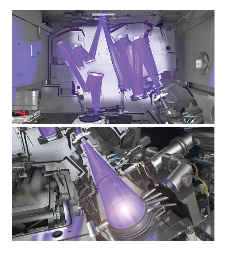
Artist's rendering of the full optical path of an EUV scanner, which uses 13.5-nm wavelength light for semiconductor lithography **(top)**. Artist's rendering of an EUV source, which at 13.5-nm wavelength is invisible to the eye but crucial to production of advanced semiconductors **(bottom)**. Courtesy of ASML.
