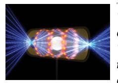
This artist's rendering shows an NIF target pellet inside a hohlraum capsule with laser beams entering through openings on either end. The beams compress and heat the target to the necessary conditions for nuclear fusion to occur. Ignition experiments on NIF will be the culmination of more than 30 years of inertial confinement fusion
