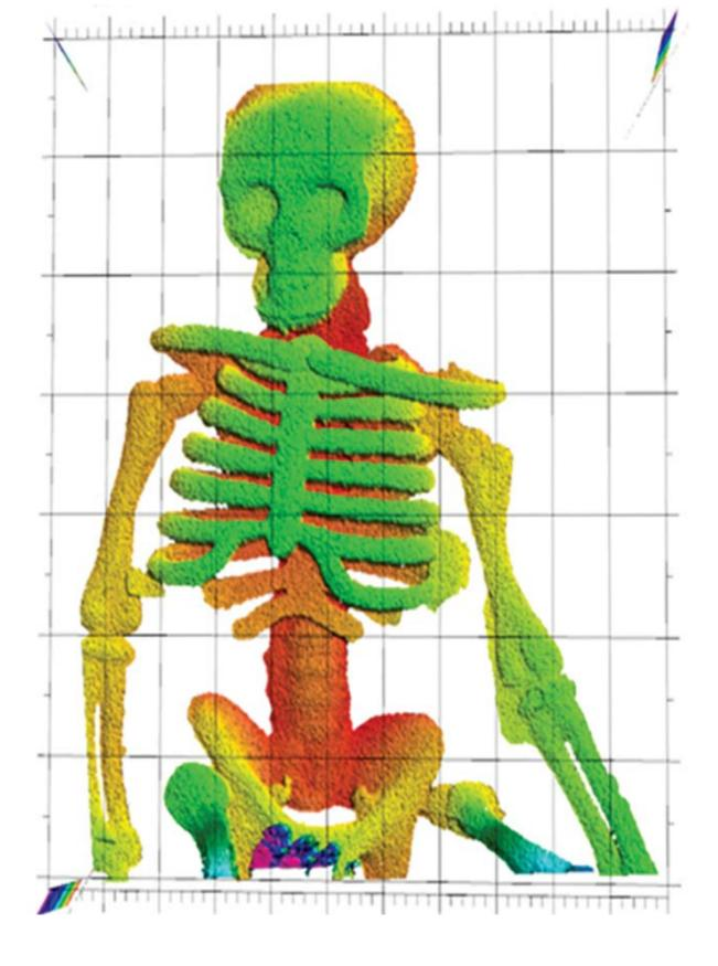
NIST researchers demonstrated that laser ranging could "see through flames" to make this image of a plastic skeleton toy. Laser ranging captured the skeleton's complex 3D shape, with depth indicated by false color. The plastic did not melt or deform in the fire, unlike pieces of chocolate. Courtesy of Baumann/NIST.
