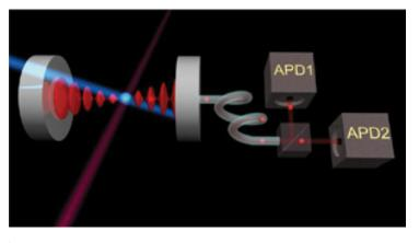
A high-finesse optical cavity consisting of two mirrors traps and accumulates the photons emitted by the ion into a mode. The ion is excited cyclically by an external laser and at each cycle a photon is added to the cavity mode, which amplifies the light. (University of Innsbruck © Piet Schmidt)
