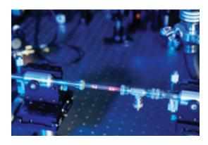
Extreme nonlinear optical techniques have succeeded in upconverting visible laser light into x-rays, making a tabletop source of coherent soft x-rays possible. (University of Colorado)
