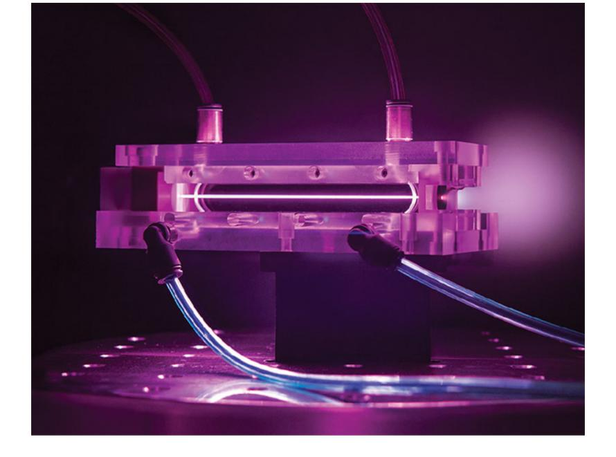
Experiments with a 9 cm-long capillary-discharge waveguide used in BELLA (the Berkeley Lab Laser Accelerator) generate multi-GeV electron beams. The plasma plume is made more prominent with HDR photography. Courtesy of Roy Kaltschmidt and Lawrence Berkeley National Laboratory/2010 The Regents of the University of California, through the Lawrence Berkeley National Laboratory.
