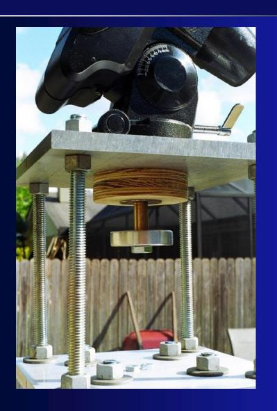
I used the plug left over from cutting the hole in the upper plate to accept the mount, to build the tie down. Using that disc of aluminum, a 10 mm bolt and other odd pieces, I fashioned a hand tightened spanner to mount my CG5 German Equatorial Mount to the plate assembly.
