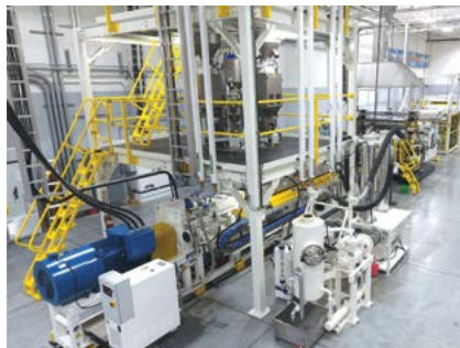
PTi's new HVTSE® dryerless sheet extrusion demo system complete with material handling thru 2-up winding provides Laminex a quick, high quality entre' into PET sheet markets.
