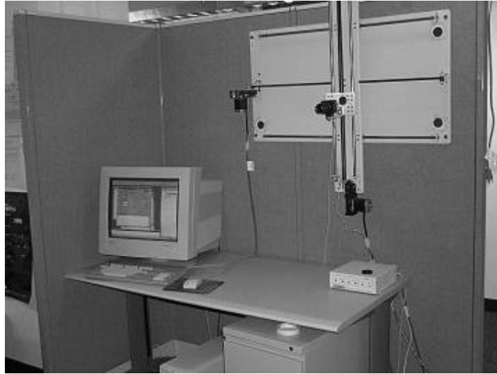
Figure 1-4 Computer controlled X-Y platform and digital camera.
