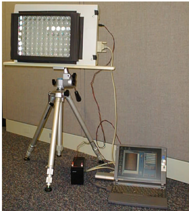
Figure 3-1 Low cost light field capture device.
