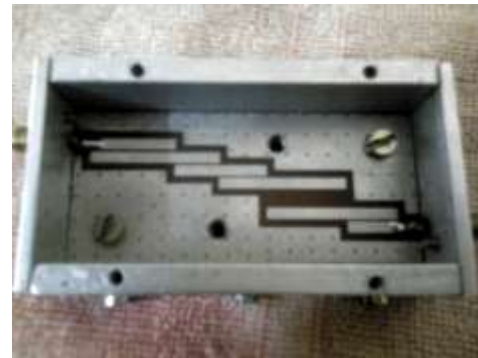
Fig. 8 Fabricated microstrip parallel coupled line band pass filter
