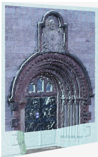
Figure 11. Registration of the reconstructed point cloud onto the ground truth data ( Herz-Jesu-K7 stereo-pair).
