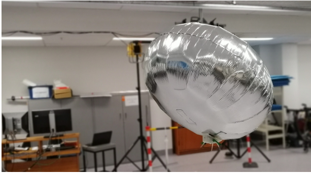
FIGURE 1. The proposed low-cost, open-source, indoor robotic airship. The airship consists of a gondola containing all the electronics and rotors and a Qualatex Microfoil balloon (metallised PET).
