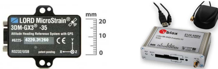
Fig. 1. Microstrain 3DM-GX3 - 35 (on the left) and Ublox EVK-M8T (on the right).
