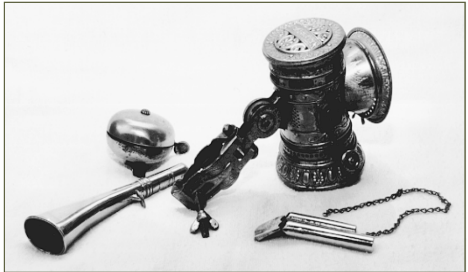
Bicycles were quiet and often startled pedestrians and horses. Laws or ordinances were passed that required one or more of these warning devices, all made in the mid-1890s to the early 1900s: (left to right) English horn, lever bell, “Search Light” lantern, and “Duplex” whistle which had two tones. Carter Collection.
