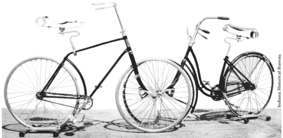
A pair of 1892 Columbia spring fork light roadster safety bicycles from the Carter Collection. Note the differences between the men's frame (left) and the women's frame (right).
