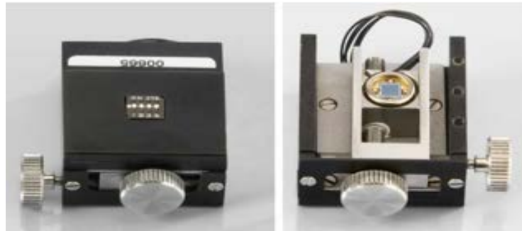
Figure 1.2 Detector assembly, top view (left) and bottom view (right). 4
