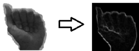
Figure 5. Applying Morphological Gradient Transform
