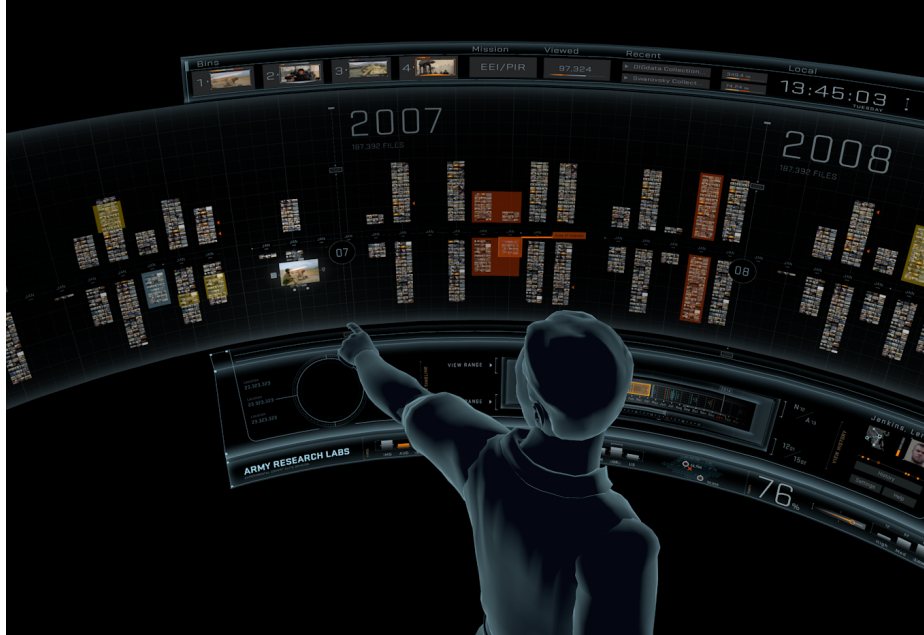
Fig. 1. Over-the-shoulder view of the VIE and a user viewing a photo collection based on time. The timeline graph shown can be zoomed in to see that each part of the graph is composed of the images taken during that part of the timeline. The images are framed on the top and bottom by the non-moving VIE console.
