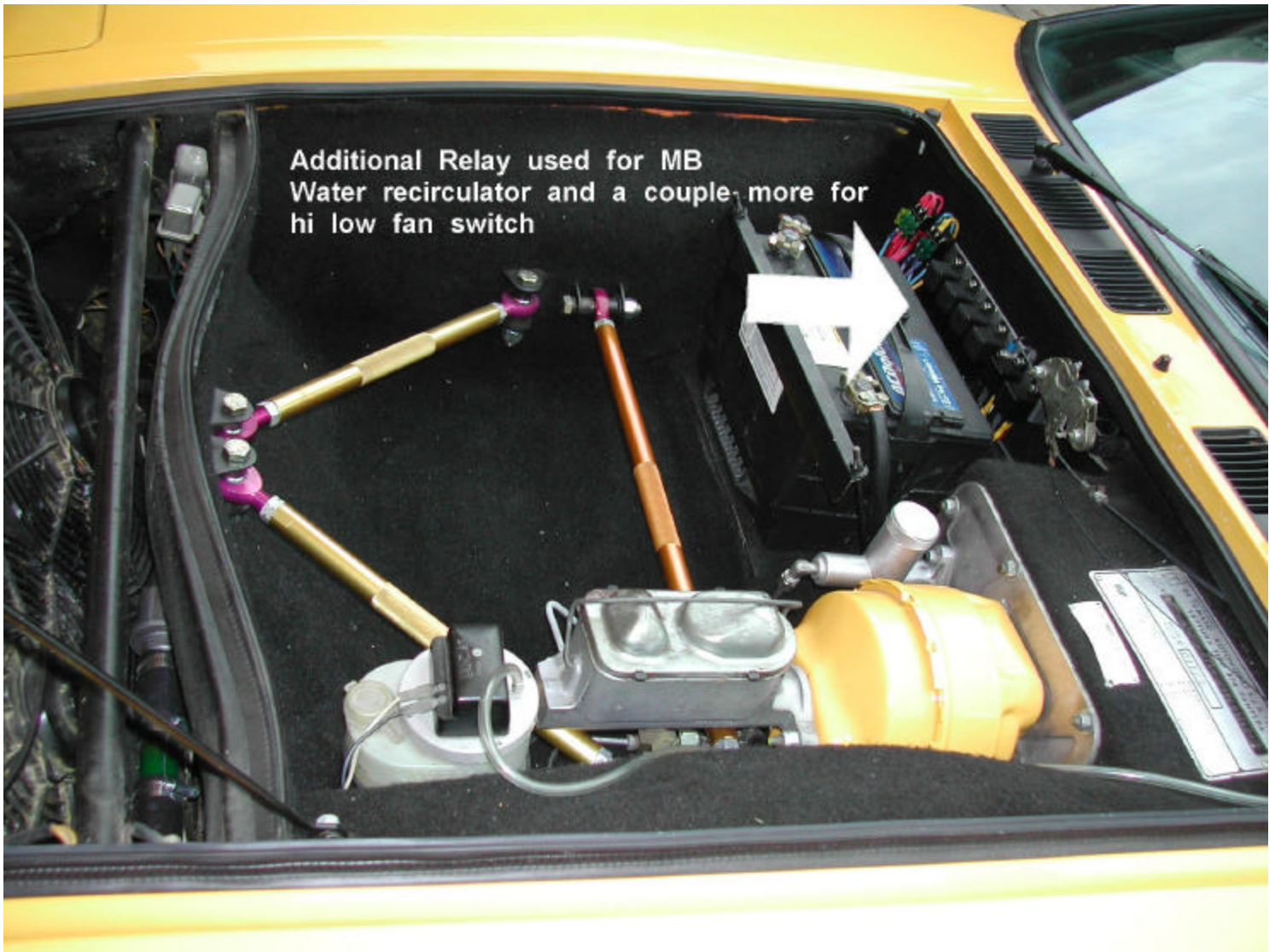
I wired the pump to the additional relay on my Rick Moseley kit. When energized, the pump circulates coolant via a hose that passes through the forward bulkhead and connects to the stock heater control valve prior to the core.
