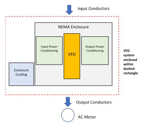
A conceptual diagram of a VFD system is shown in Figure 1.
