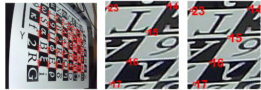
(a) Detected grid points (b) Before fine tuning (c) After fine tuning
