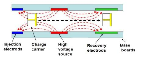
Figure 2 : Schematic Layout of A basic unit of the New Electrostatic Generator
