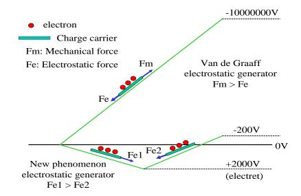
*Figure 3* : Schematic Explanation of the Principles behind the Two Electrostatic Generators
