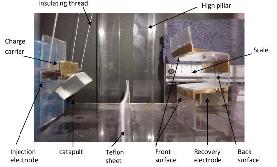
Figure 4 : A Photograph of the Main Part of the Experiment Equipment of the New Electrostatic Generator
