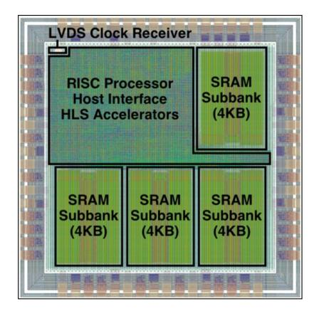
BRGTC1 in 2016 RISC processor, 16KB SRAM HLS-generated accelerator
