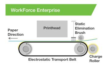
The WorkForce Enterprise uses an electrostatic transport belt that ensures the paper is completely flat, enabling the smoothest of gradients and consistently sharp images.
