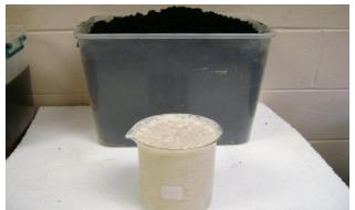
Terephthalic (TPA) acid produced after treatment with stoichiometric amounts of acid.
