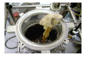
Picture 3 Fabrics are removed from reactor dried after squeezing out reagent and rinsed with water.
