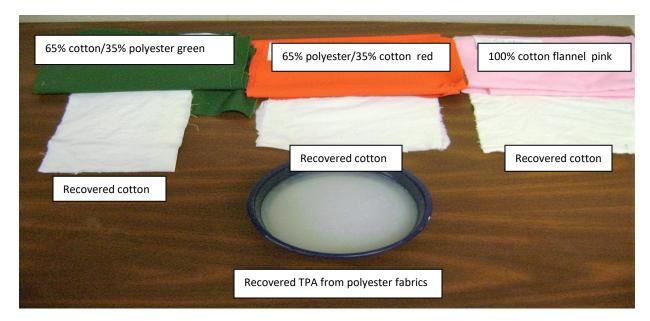
The dyes in these fabrics were completely removed along with PET within 20 minutes in the reagent at temperatures of 100-110° C. Samples were retested to confirm that PET was completely removed. The Terephthalic acid resulting from the depolymerization of PET is shown below in the dish.
