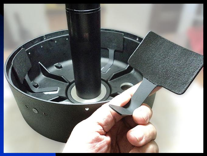
By coating each contact pad with a spray-on rubberized coating, only light contact pressure is needed to effectively lock the mirror.
