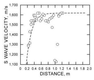
Figure 16. Block 1 MVP velocity vs. distance from blasthole.
