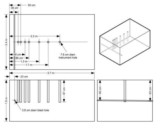
Figure 10. Engineering drawing of block 2 blasthole and strain gage sensor locations.
