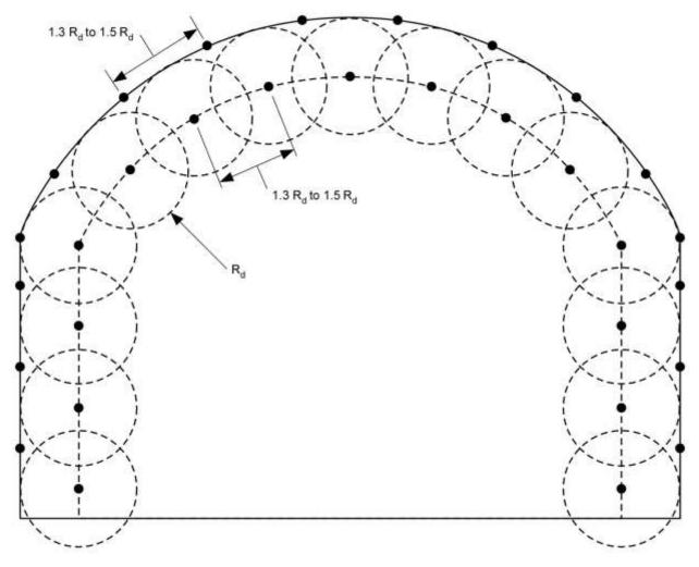
Figure 27. Buffer row hole locations, buffer hole practical damage circles, and perimeter holes at the cusp locations.
