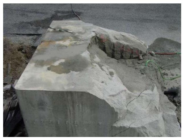
Figure 14. Block 3 during wire sawing to expose radial fractures.
