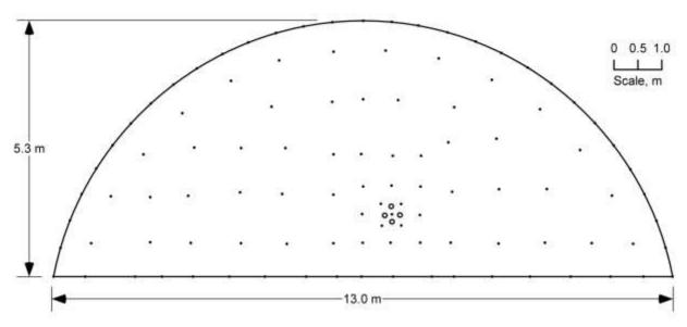
Figure 34. Example of the successful railway tunnel blast design in Spain.
