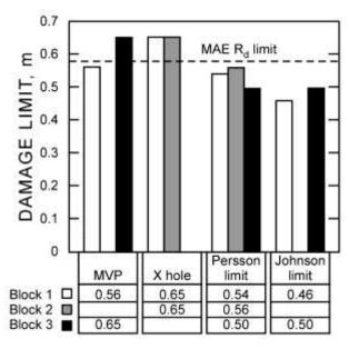
Figure 26. Summary of damage limit results of block experiments compared to MAE R<sub>d</sub>.
