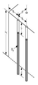
Figure 7. Isometric view of Ash's blast design parameters [Ash 1963a,b,c,d].
