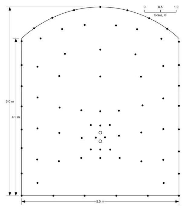
Figure 32. Example of the successful blast design in Sweden with decoupled perimeter cartridges.
