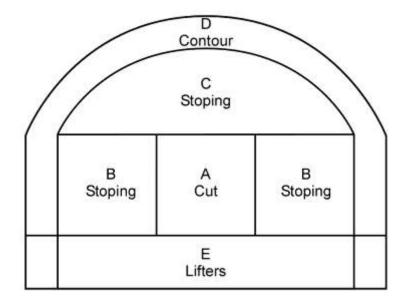
Figure 1. Diagrammatic representation of the design sectors involved in a drift round. After Holmberg [1982].
