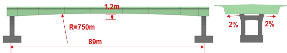
Fig. 1. The construction layout of the L7 span of Dongfeng avenue freeway viaduct
