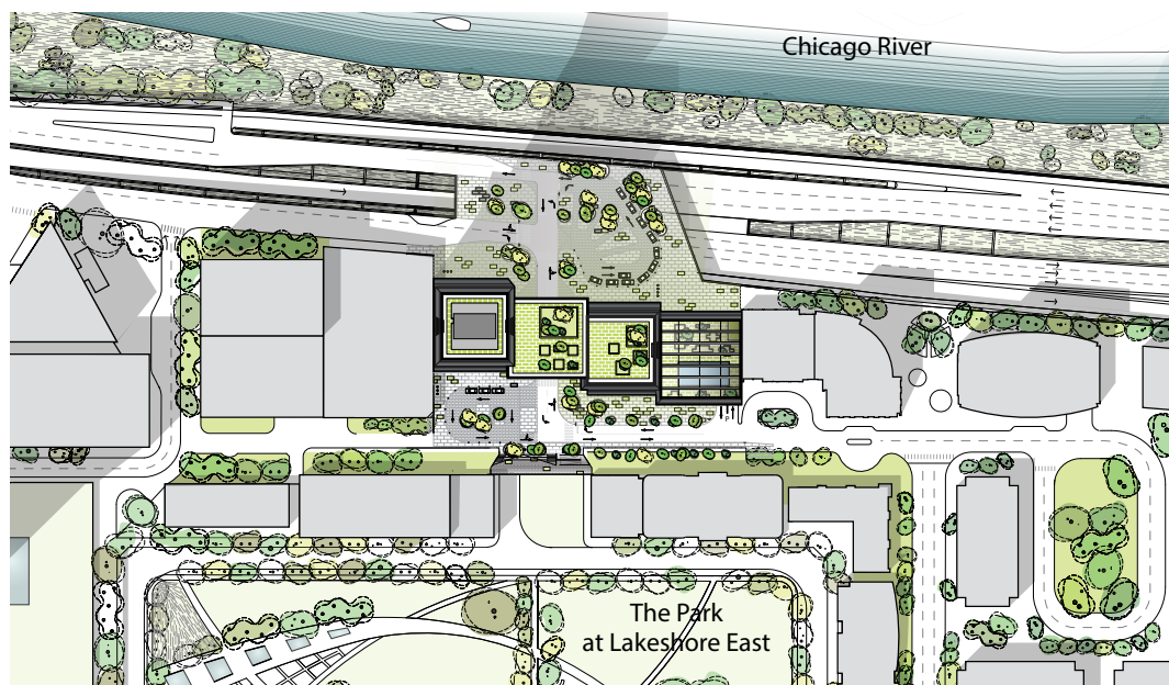
Figure 1. The building is composed of four volumes, which allows the massing to adjust to the site's geometry, while creating a generous entry plaza on the northeast and southwest sides of the building.
