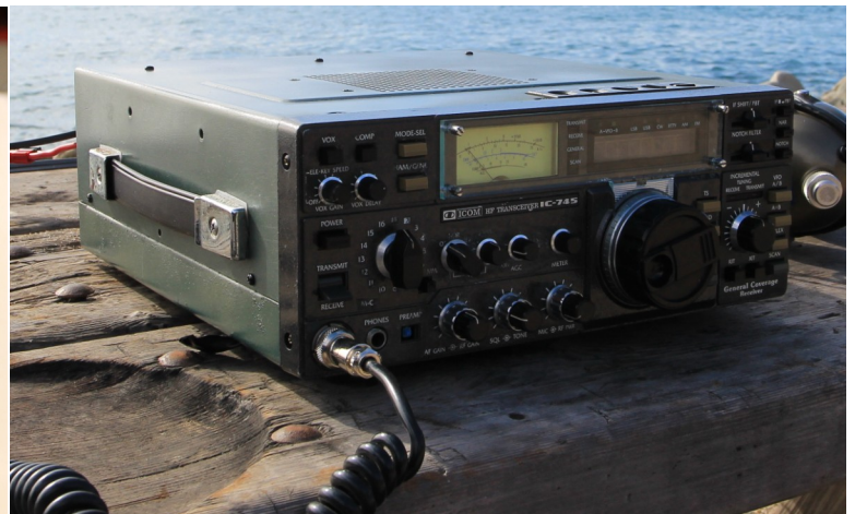
After: The (Almost Fully) Restored IC-745
