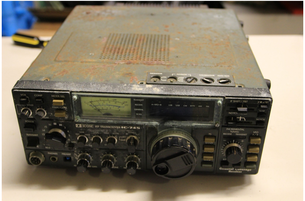
Before: Icom IC-745 with major corrosion
