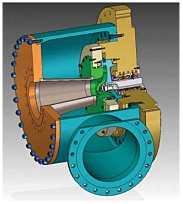
Figure 7 – SSNE SINOPEC 4MW Euler Turbine Generator Project
