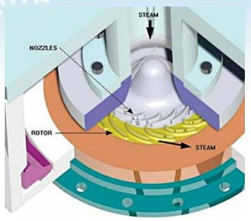
Figure 1 – Microsteam Turbine Operation
