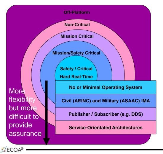
OMCOS\* found that loosely coupled Service-Orientated Architectures (SOA) and Publisher-Subscriber are important concepts that can provide the flexibility needed in increasingly complex, ad-hoc, networked systems
