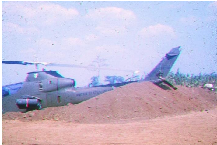
HUEY COBRA AT ANDERSEN WITH ITS TAIL ROTOR KNOCKED OFF BY AN EMPTY PLASTIC DRUM BLOWING ABOUT IN THE MAIN ROTOR WASH Photo: Sapper Brian Hopkins 3 Troop
