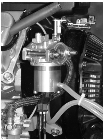
Figure 15. Prototype PCI fitted to the throttle body of an 80cc engine.
